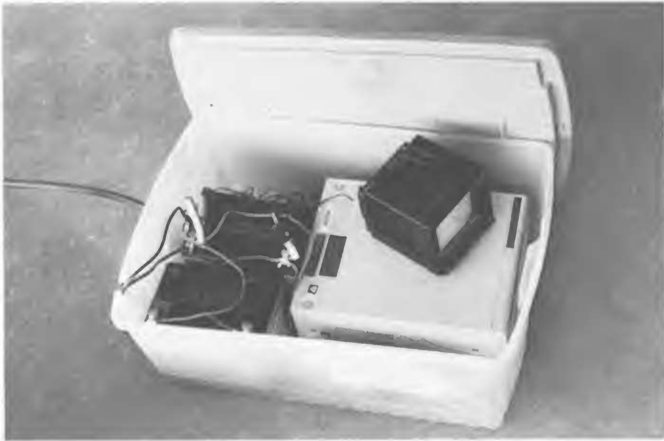
Figure 4. Weatherproof, rubberized bin housing video recorder, batteries for powering entire system, and spare tapes, with a portable monitor used temporarily to check video image reception and quality.
